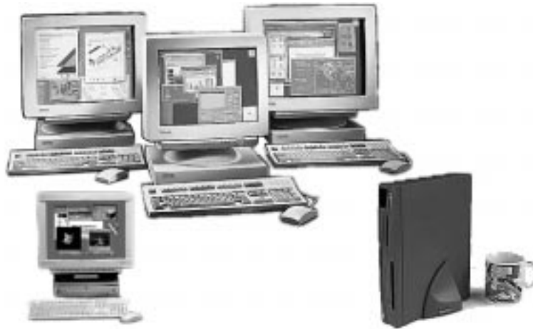
Figure 4.5: Desktop Network Computers: The Tektronix NC200 Series[34] (top left), the NCD Explora 400[14] (bottom left) and the DEC StrongARM™ Reference NC[10] (bottom right)
